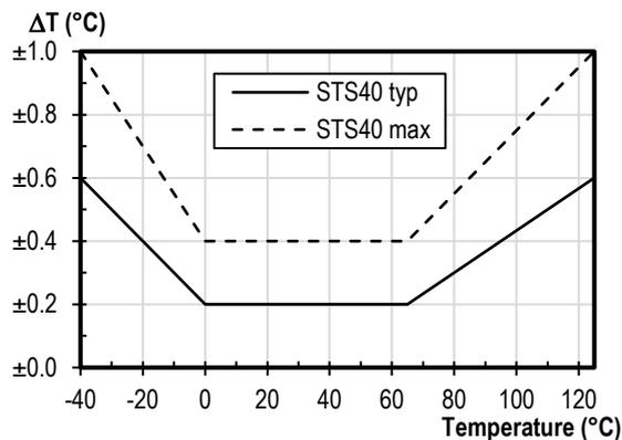
**Figure 2.** STS40 typical and maximal temperature accuracy.
