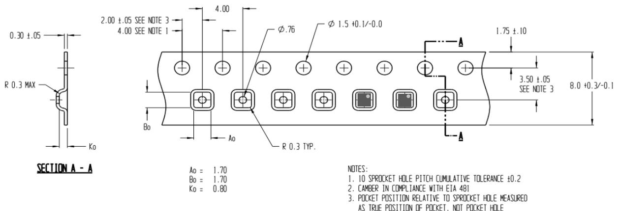
**Figure 7.** Tape and reel specifications including a depiction of two sensors in their corresponding pockets. In this orientation, Pin 1 is in the upper right corner, as indicated by the dot on the sensor and in the drawing.
