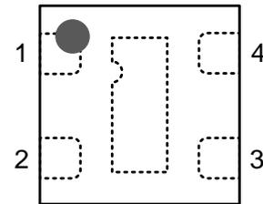
**Figure 6.** Pin assignment (transparent top view). Dashed lines are only visible if sensor is viewed from below. The die pad is not directly connected to any pin. Pin-1 is indicated by the cutout of the die pad from the bottom side (see dashed lines) and the top side laser marking (dot in upper left corner).
