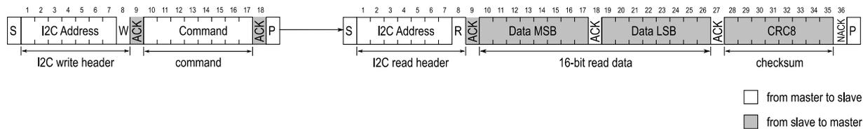
**Figure 3.** I<sup>2</sup>C transfer types: First a write header is sent to the I<sup>2</sup>C slave, followed by a command, for example “measure *T* with highest precision”. After the measurement is finished the read request directed to this I<sup>2</sup>C slave will be acknowledged and transmission of data will be started by the slave.
