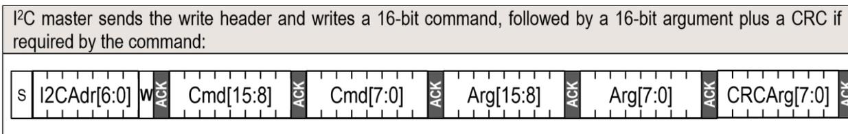
**Figure 2:** I<sup>2</sup>C sequence to send a command with an argument to the sensor.
