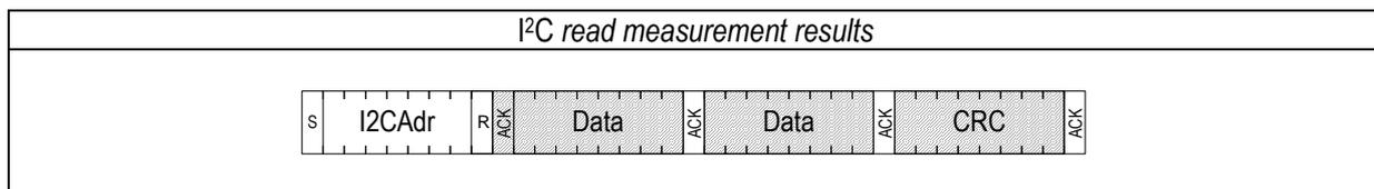
The CRC byte is calculated using the generator polynomial  $G(x) = x^8 + x^5 + x^4 + 1$  (hex 0x31). The initial value is 0.
