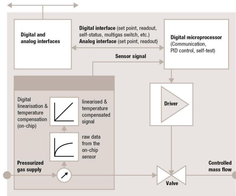
Figure 2: Block diagram CMOSens® SFC5400 mass flow controller.
