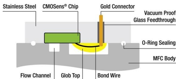
Figure 7: Vacuum tight glass feed through (longitudinal view)
