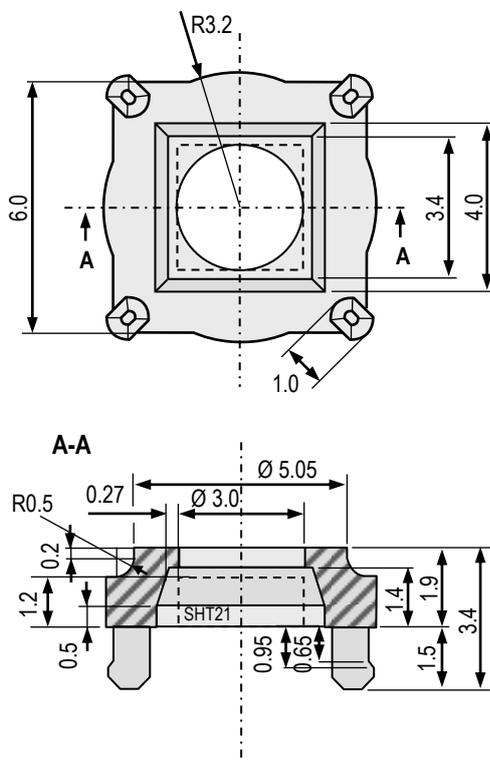
**Figure 1:** Drawing of the filter cap SF2 (body only). Dimensions are given in mm (1mm = 0.039inch), tolerances are  $\pm 0.1$ mm. Add 0.15 to total height due to the filter membrane. The cavity inside the cap fits to SHT2x/3x/4x, SHTC1 and SHTC3 sensors. Additional space for solder joints are left open around the sensor.
