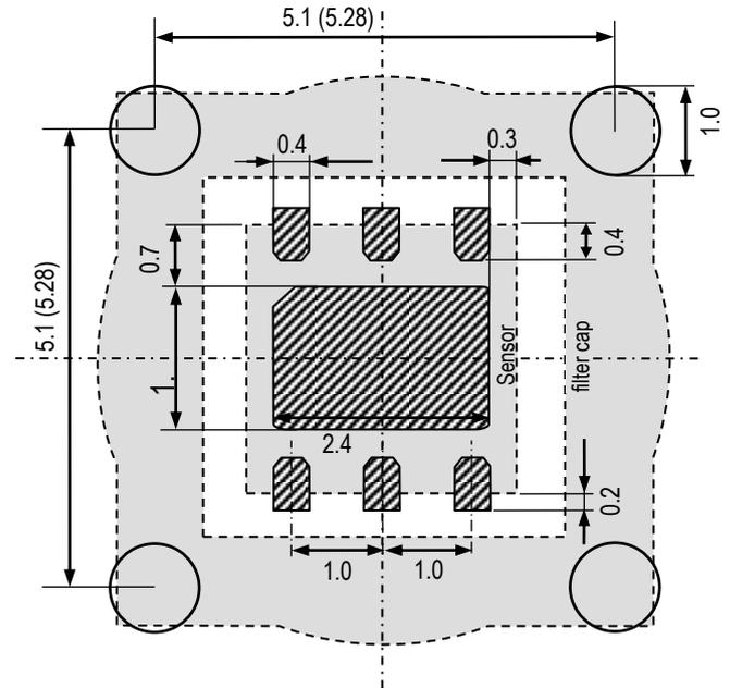
**Figure 3:** PCB layout example of SHT2x and filter cap SF2; all DFN sensors of smaller size to be placed according to the example in the center of the SF2 outline. Dimensions are given in mm (1mm = 0.039 inch). The distance of the openings is 5.1mm  $\pm$  0.05mm if the sensor should clip on the PCB and 5.28mm if the pins are used for adjustment only. By varying the openings distance about  $\pm 0.05\text{mm}$  the clipping force may be adjusted.
