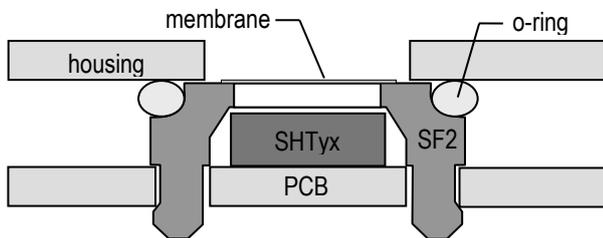
**Figure 2:** Side view of SF2 filter cap mounted between PCB and housing wall. The volume below the membrane is kept minimal and the membrane is separated from the surrounding volume enclosed by housing.
