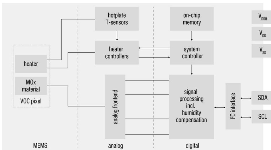
**Figure 1** Functional block diagram of the SGP40.
