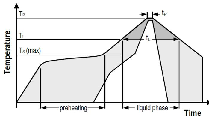
**Figure 15** Soldering profile according to JEDEC standard. Recommended conditions are  $T_P = 245\text{ }^\circ\text{C}$  and  $t_p \leq 30\text{ s}$  for Pb-free assembly,  $T_L < 220\text{ }^\circ\text{C}$  and  $t_L < 150\text{ s}$ . Ramp-up rate  $<3\text{ }^\circ\text{C s}^{-1}$  and ramp-down rate  $<4\text{ }^\circ\text{C s}^{-1}$ .
