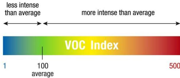
**Figure 8** Explanation of the VOC Index scale.
